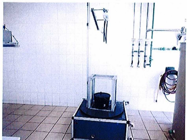
picture 4 EUT no.1 with mounted holder on the turn table before the water jets test IPX5
