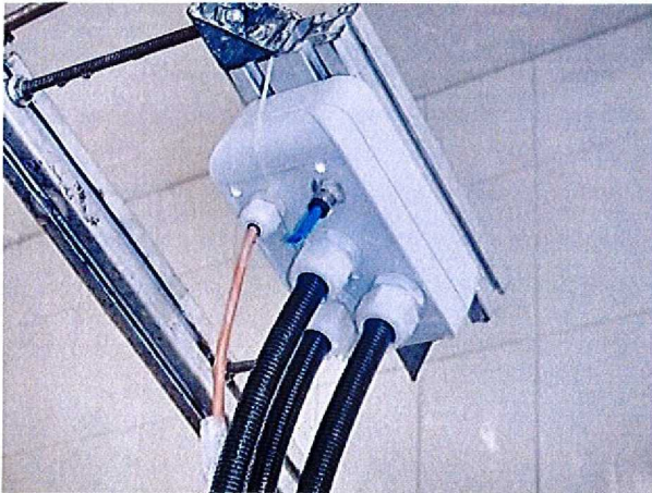
Picture 7 EUT no.1 mounted on the holder after the water jets test IPX5
