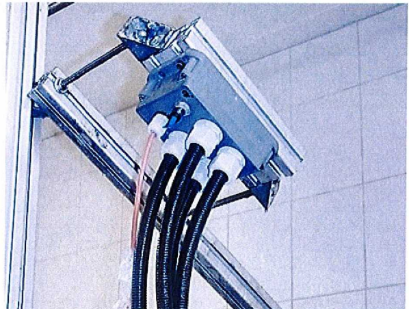
Picture 10 EUT no.2 mounted on the holder after the water jets test IPX5
